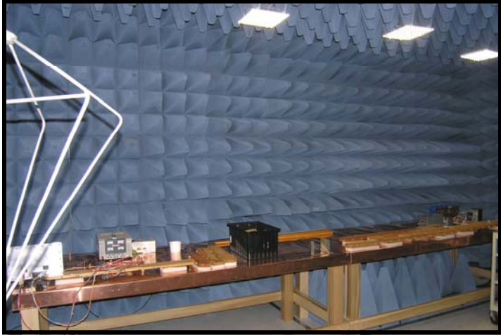
MIL 461 / DO 160 Anechoic Chamber Polyurethane Absorbers
